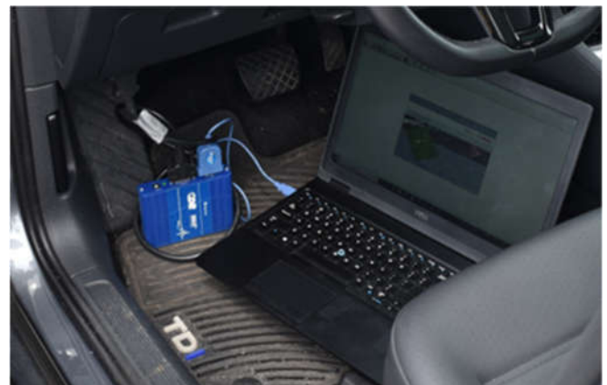
Figure 2. EDR data imaging using a Bosch CDR interface
