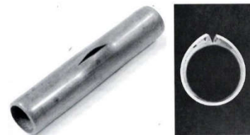
Figure 5. Cooper water pipe fracture due to over-pressure event
